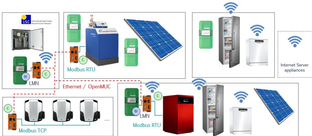
Figure 12: Implementation of ICT for appliance control in SoLAR
